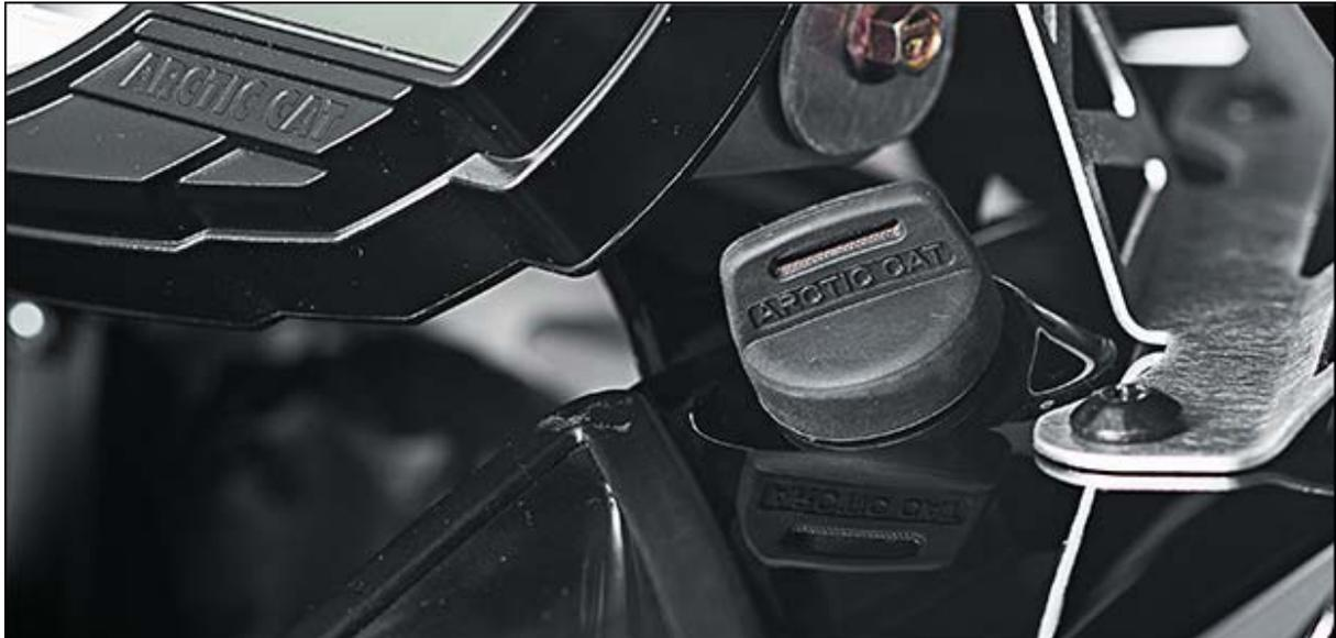
Picture 3: The ignition key is located on the right side, next to the steering handle. Do only turn the key into the first position in the beginning, before turning it all the way.
