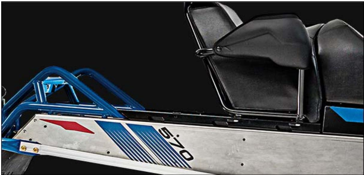
Picture 10: The tunnel rails, shown on the picture, allow you to remove the passenger seat, or add a third seat.
