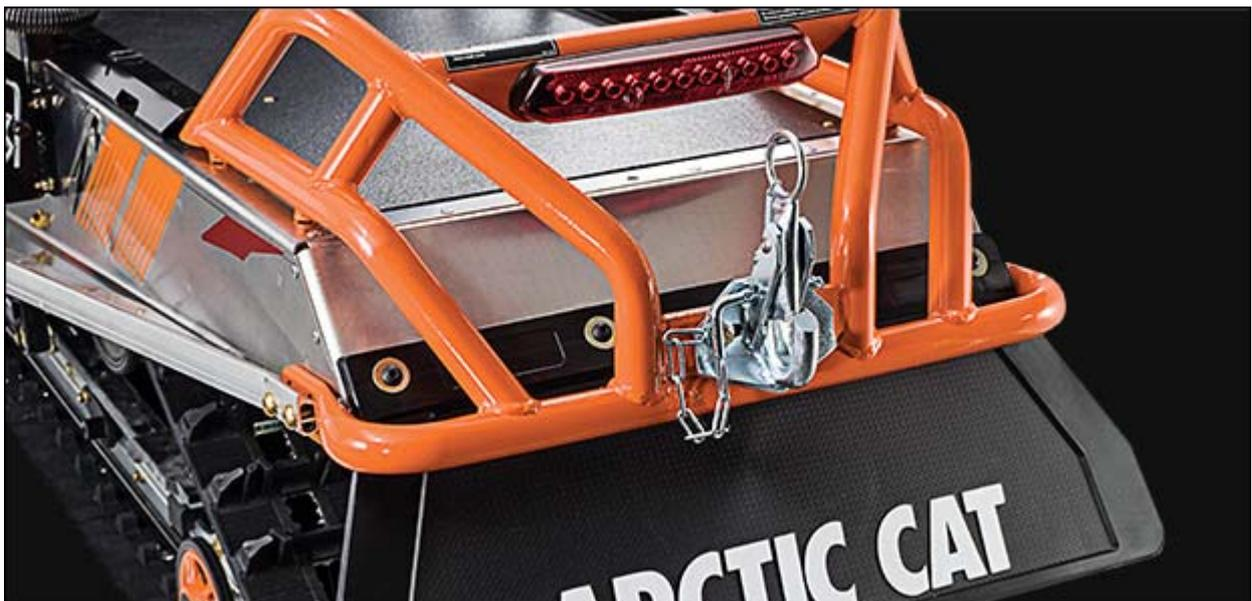
Picture 8: The snowmobile is equipped with a heavy-duty hitch on the back, so it is possible to pull a sledge.
