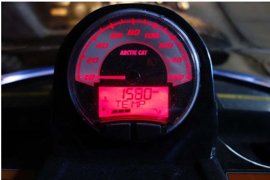
Picture 4: The text "temp" appears on the speedometer after turning on the engine. Wait for the engine to heat and the text to disappear before start driving the snowmobile.
