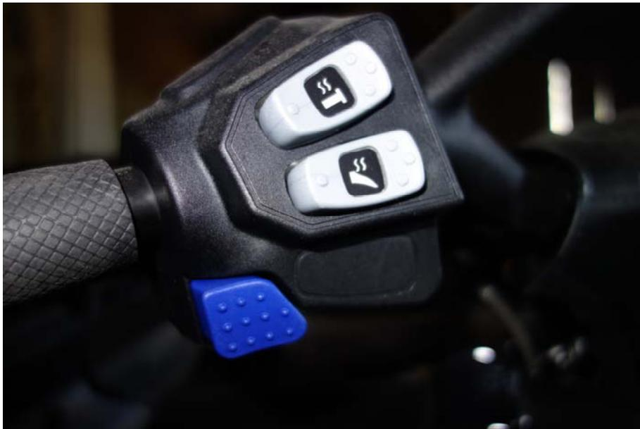
Picture 7: For turning on the heat in the steering-handle and the for the feet pres the grey buttons on the left steering-handle. The button on top is for the hands, and the button below is for the feet. In neutral position (middle) there is no heat, while to the left (1 dot) is minimum heat, and the right position (3 dots) is maximum heat.
