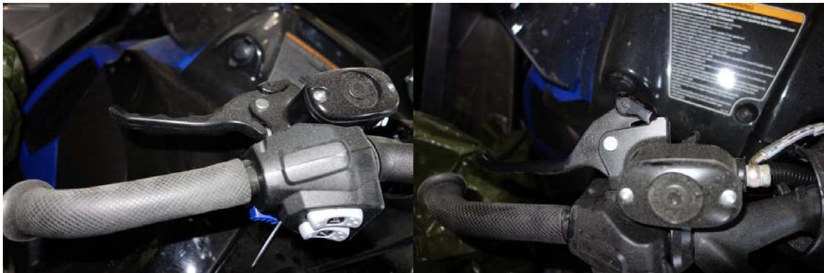
Picture 1: The brake is in the “un-locked position” to the left, and in the “locked position” to the right.
