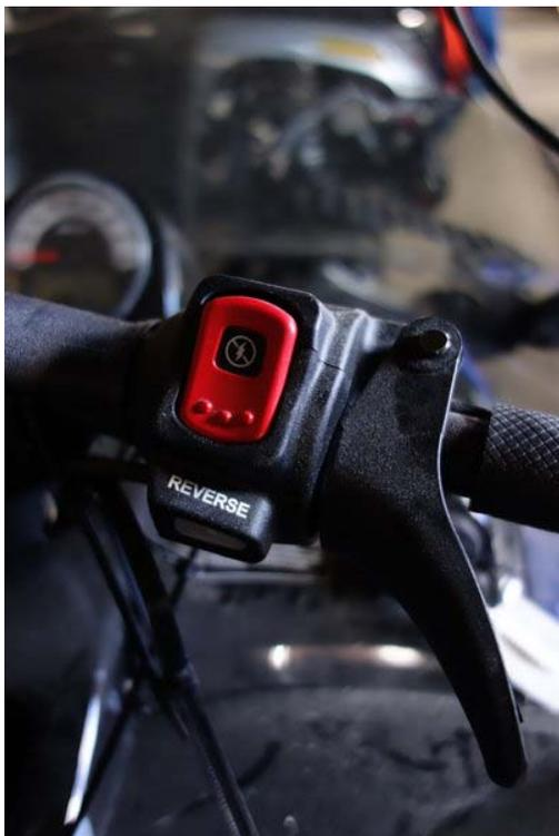
Picture 2: To turn on the electricity of the snowmobile, press the red button down into this position.
