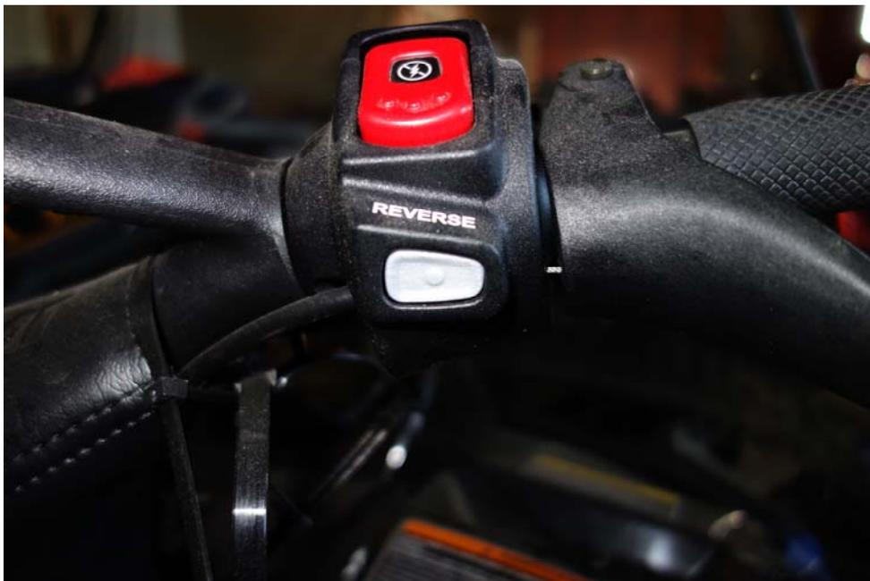
Picture 6: The snowmobile has a “Push-button reverse”. To go backwards, just push the grey button shown on the picture above.
